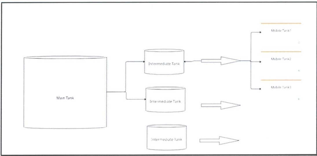
The main and intermediate tanks will be granted by connected gauging system that transmit the information to the facility control room. The gauging and sensor installed need to consider the volume, density and temperature. The software need to incorporate the VCF (Volume correction factor) formula in accordance with the MOEW standards.
